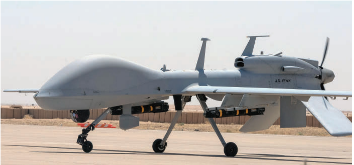
An MQ-1C Gray Eagle unmanned aerial system, equipped with 3rd Gen FLIR sensors prepares to conduct a mission from Al Asad Air Base, Iraq
